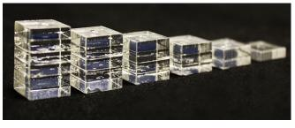
Figure 14: Calibration pattern to determine laser power for welding up to six layers of acrylic.
