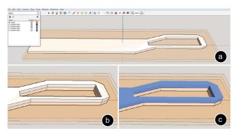
Figure 9: (a) Sketch scissors outline, use *pull* tool to extrude to first scissor outline, then (b) second scissor outline. (c) Use *loosen* tool to disconnect both layers.
