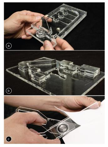
Figure 1: LaserStacker produces laser cut objects consisting of multiple layers of acrylic without requiring manual assembly: It assembles the object by not only cutting with the laser, but also welding, and healing the cut. Three example objects: (a) a pinball table with spring (10 min), (b) an architectural model of our university campus (7 min), and (c) a simple but functional pair of scissors (3 min).
