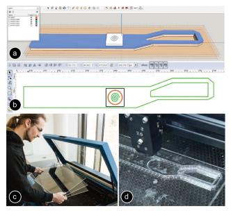
Figure 2: Creating the scissors with LaserStacker.
