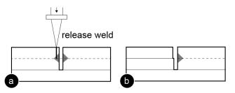
Figure 7: Releasing a weld: (a) creating a new cut in very close proximity, (b) the material evaporates and releases the weld.
