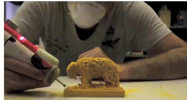
**Figure 3.** FreeD is a hand-held mill that guides the user through fabrication based on a pre-selected digital model.
