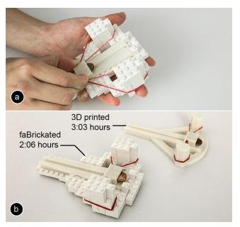
Figure 15: (a) A faBrickated penny ballista takes (b) only 2:06h for printing and 11 minutes for assembly compared to 3:03h when 3D printing entirely.
