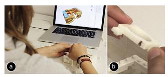
Figure 5: (a) Assembly instructions highlight the next brick in blue. (b) Each 3D printed part has a unique ID.
