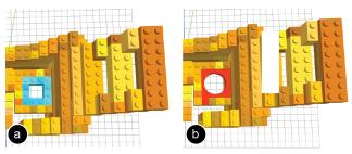
Figure 4: Using the *high-res* brush the user defines the region that will be 3D printed in full detail.
