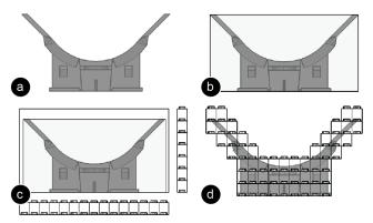
Figure 10: Legofying: (a) model, (b) bounding box, (c) extended bounding box, (d) legofied model.
