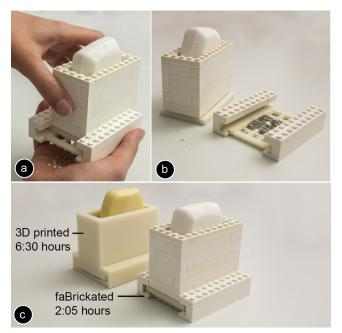
Figure 14: (a,b) This soap dispenser only takes (c) 2:05h and 5 minutes assembly compared to the 6:30h of traditional printing.
